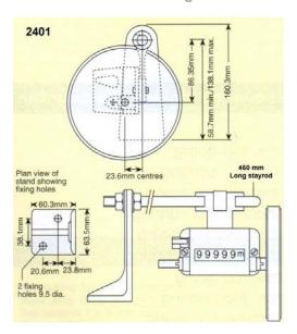
This rugged instrument has a wide range of applications where an accurate record of length is required. It is a strong, heavy duty unit for use on calenders, tenters, rolling, ribbon winding textile machinery and almost all other continuous manufacturing processes.
