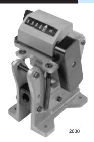
This robust machine measures the length of wire and other materials up to 15mm (0.59in) diameter. The 250mm circumference, precision ground measuring wheel runs in self lubricating bearings.
